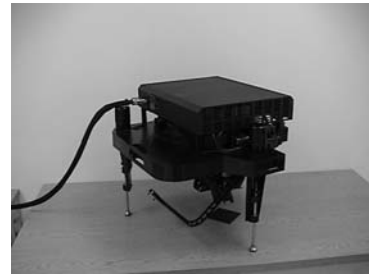
Figure 1.0-1. The scatterometer used to acquire the data
