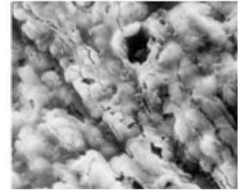
Microscopic view of surface pores in anodic coating.
