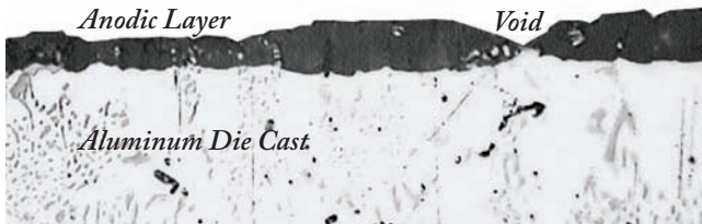
Figure 2 – Cross-section of an aluminum die cast part reveals the irregularities in the anodic coating layer. Voids, or areas of little or no coating, occur due to the migration of silicon or other non-aluminum particles. These areas are particularly vulnerable to corrosion and coating failures. Image captured at 500x magnification.
