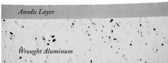
Figure 3 – Cross-section of a wrought aluminum part reveals an extremely uniform anodic coating. A uniform coating minimizes areas of vulnerability and offers the best protection.
