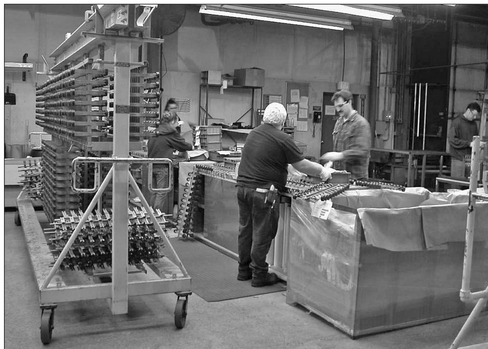
Pioneer Metal Finishing team members use specialized fixtures to process customer parts.
