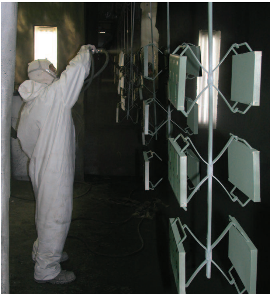
A spray operator manually applies powder coating on the plant's combination liquid-powder coating line.
